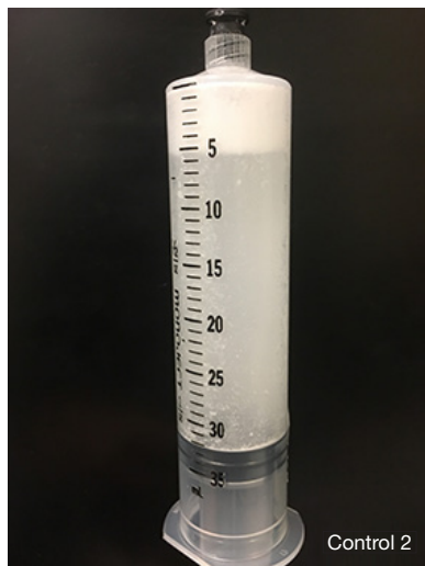
Figure 3 Control 2 in a 35 mL syringe showing the majority of crystals have floated to the top.
